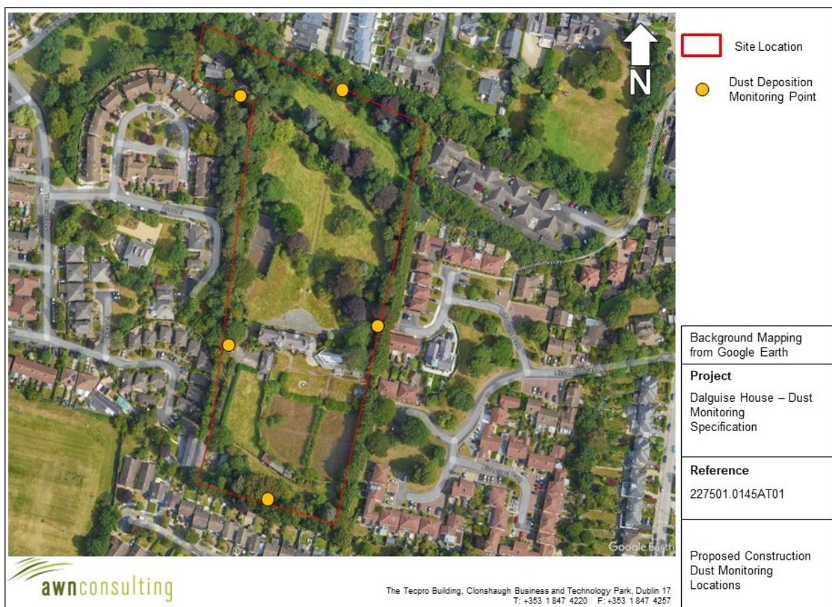
Figure 12 – AWN Consulting Ltd Proposed Construction Dust Monitoring Locations
